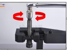
The tightening torque of the nozzle cap must be installed in accordance with the tightening torque specified in the injector maintenance manual
