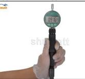
If the value is greater than normal, thicken the gasket for oil-nozzle needle valve lift adjustment; if the value is less than normal, reduce the gasket for oil-nozzle needle valve lift adjustment
