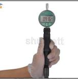
If the value is greater than normal, thicken the gasket for oil-nozzle needle valve lift adjustment; if the value is less than normal, reduce the gasket for oil-nozzle needle valve lift adjustment
