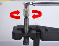
The tightening torque of the nozzle cap must be installed in accordance with the tightening torque specified in the injector maintenance manual
